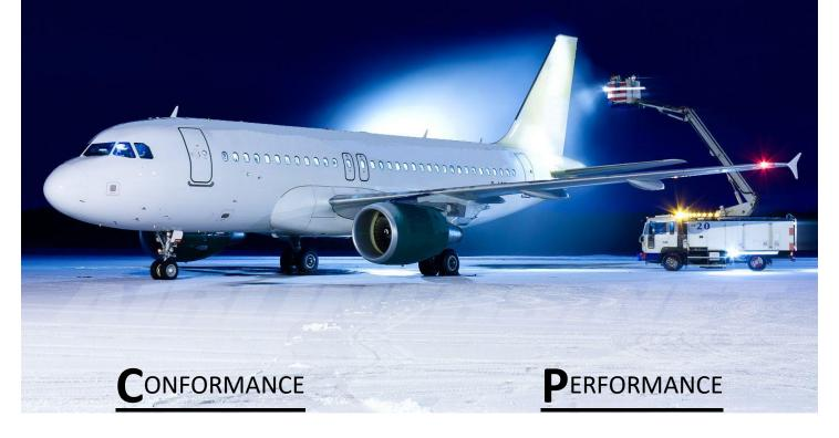
AllClear Systems' Lift-Off P-88 Type I product, is certified to SAE AMS 1424/1; the international performance and certification specification for aircraft deicing fluids.
