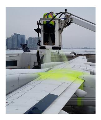
Proper and uniform coverage should be ensured by applying a sufficient quantity to completely remove any remaining Type I fluid. Aircraft surfaces should be coated to a depth of 1 to 3 millimeters. Insufficient application will result in a thin layer and reduced holdover protection.
